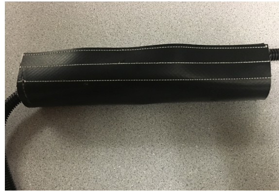
Step 2: Securely wrap the two ends of the protective sleeve together making sure velcro is sealed on the top side of the front jump start plug holder.
