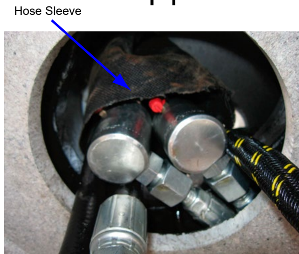
Photo taken looking up from the crane box. Image is for illustrative purposes only, actual crane installation may vary. The pressure, return, and rotation hoses are wrapped in the hose sleeve.
