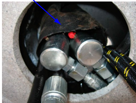
Photo taken looking up from the crane box. Image is for illustrative purposes only, actual crane installation may vary. The pressure, return, and rotation hoses are wrapped in the hose sleeve.
